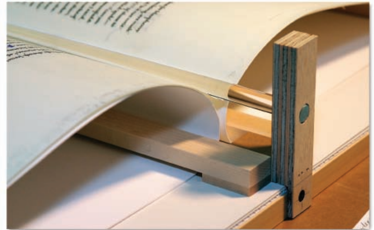
The base of the folio assembly is constructed of 4-ply museum board. Wood brackets are attached to hold the pages lightly. The vellum pages themselves are not attached to the brackets but are sewn along the outer edge to sheets of 2-ply cotton mat board. Since this board touches the pages, it must be carefully sanded smooth so that no sharp edges will come in contact with the vellum pages. The edges with the sewing will be trimmed when the pages are eventually bound. The mat board holds the pages in a curved shape, approximating the open pages of a book. Photo by Donna Kelly, Minneapolis Institute of Arts.
